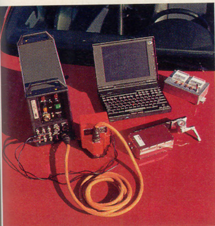
A-DAT's red box on the left became our magic box. It measured lateral acceleration independently of roll—not something every accelerometer can do. This feature allowed direct comparison between the Miata, with its noticeable body roll, and the flat-cornering Prelude. Datron's optical sensor provided the speed measurement, and the laptop computer was used to log in data.
